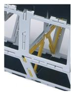
Equilateral triangles are used to create the angle of slope of the plinths. You can replace these with right-angled triangles to make the angle between the struts and the vertical 45° instead of 60°.
