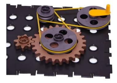
• Can you calculate how many turns of the small gear are needed to turn the large single pulley once?
