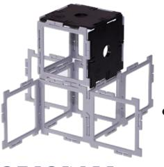
Join the housing to the support.  Now make make four strips using a double square and a single square.
